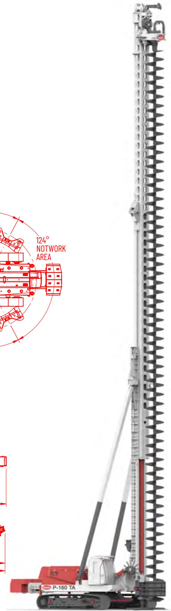
The LLAMADA **P-160TA** Piling rig is designed to facilitate without compromise the installation of continuous flight auger piles (CFA), compaction or displacement piles (FDP), secant piles(SP), continuous piles(CP)down the hole hammer (DTH), Controlled Modulus Columns (CMC) and SOILMIXING soil improvement/remediation techniques. The **P-160TA** can install piles up to **35m** deep without the need for extensions or snorkels, and from Ø 300mm up to **Ø 1.200 mm**.
