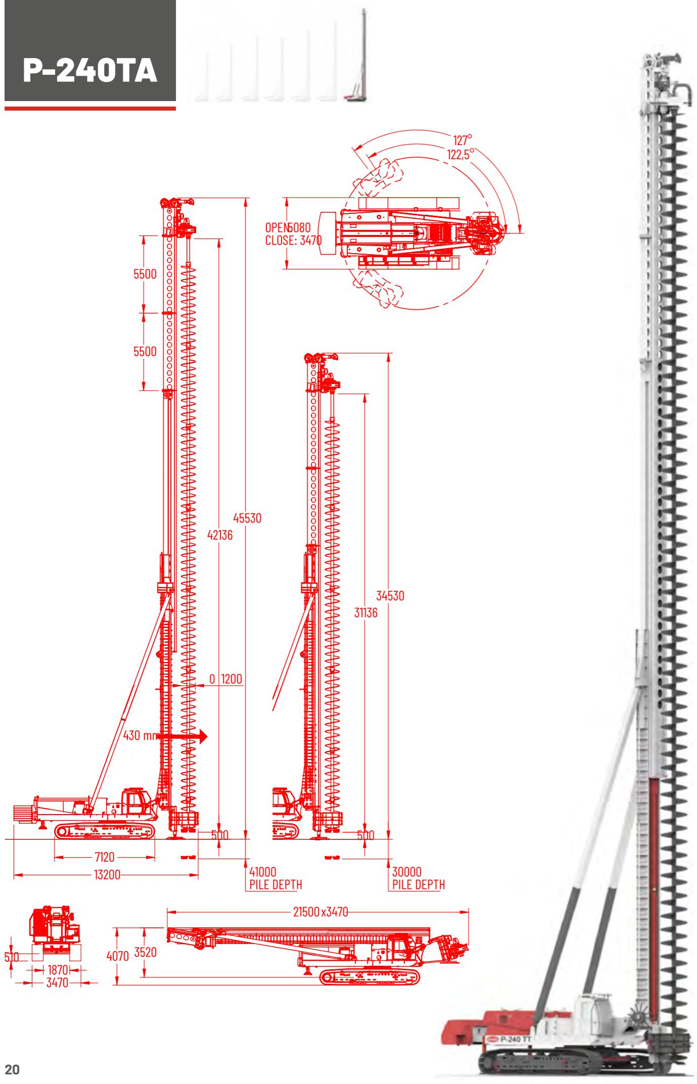
The LLAMADA **P-240TA** Piling rig is designed to facilitate without compromise the installation of continuous flight auger piles (CFA), compaction or displacement piles (FDP), secant piles(SP), continuous piles(CP)down the hole hammer (DTH), Controlled Modulus Columns (CMC) and SOILMIXING soil improvement/remediation techniques. The **P-240TA** can install piles up to **41m** deep without the need for extensions or snorkels, and from Ø 300mm up to **Ø 1.200mm**.
