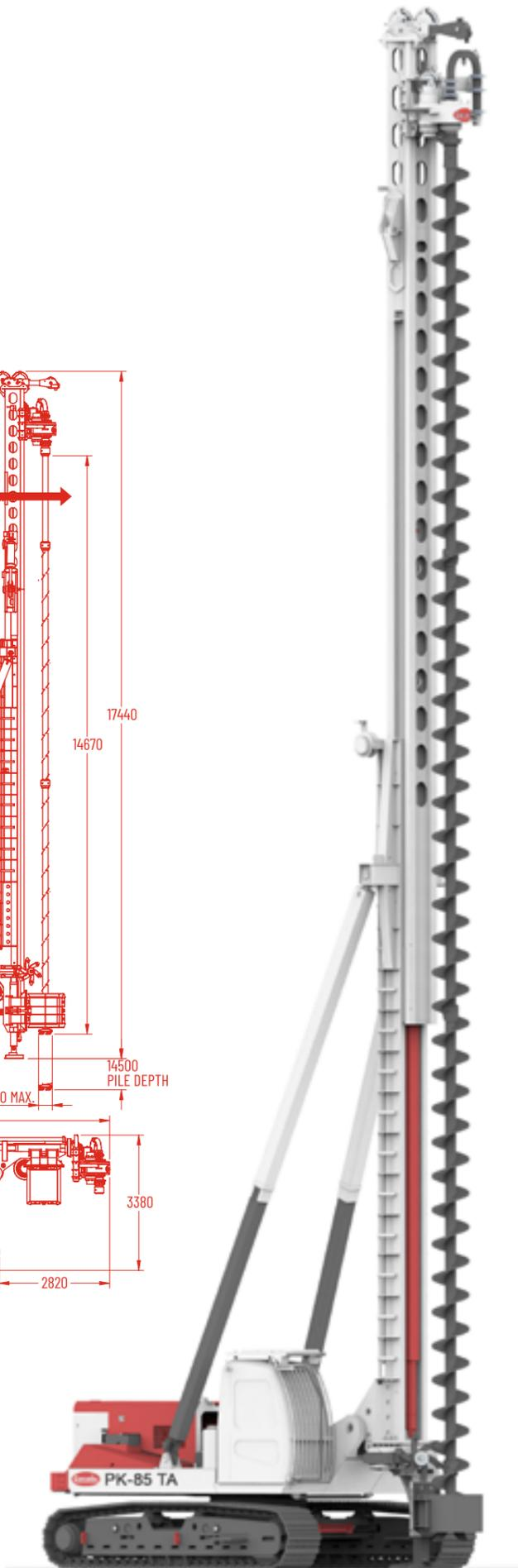
The LLAMADA **PK-85TA** Piling rig is designed to facilitate without compromise the installation of continuous flight auger piles (CFA), compaction or displacement piles (FDP), secant piles (SP), continuous piles (CP) down the hole hammer (DTH) and SOILMIXING soil improvement/remediation techniques. The **PK-85TA** can install piles up to **20m** deep without the need for extensions or snorkels, and from  $\varnothing$  300mm up to  **$\varnothing$  800mm** in diameter.
